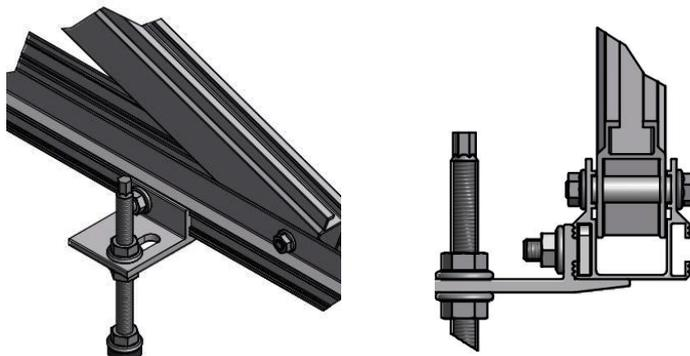
Figure 138: Fixation by universal connector
