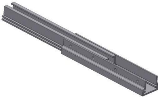
Figure 75: Insert butt connectors
