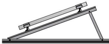
In this case, Delta supports are connected using two carrier rails (TF50/TF50+m/TF60). Modules are then mounted on said carrier rails. Please ensure that the modules have been approved for clamping on the short sides.
