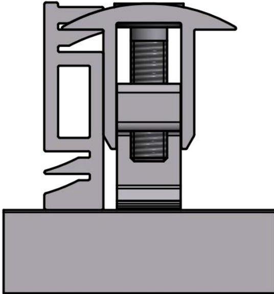
Figure 126: EC adapter with middle clamp G4
