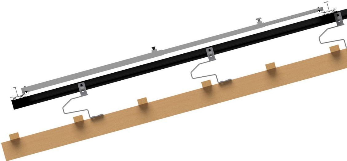
Figure 148: Positioned assembly jig
