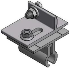
Use "Kalzip® clamps" to fasten the system on so-called Kalzip® roofs. The clamps are distributed vertically according to the number of cross girders. As a rule, fit one standing seam to each clamp. On each side the carrier rail must protrude by a maximum of 0.4 m.
