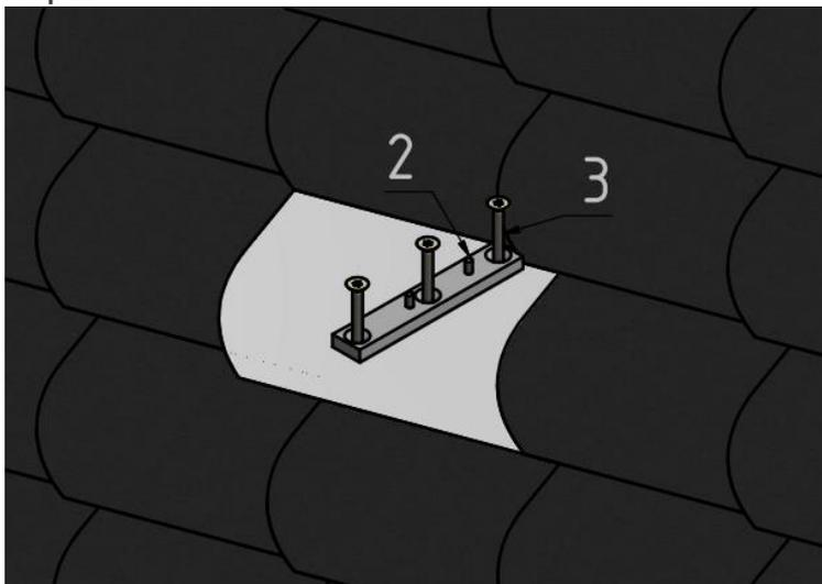
Figure 46: Fix the mounting plate
