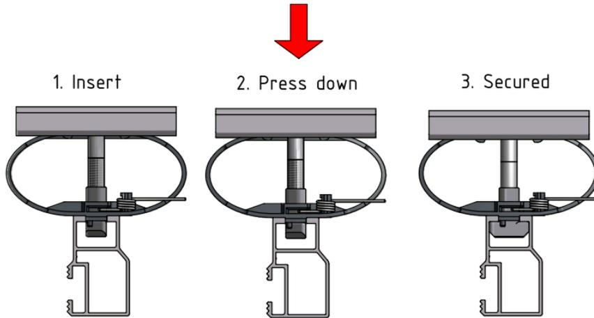
Figure 124: Inserting middle clamps G3
