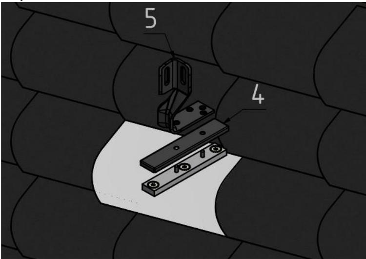
Figure 47: Cover cap and roof hook
