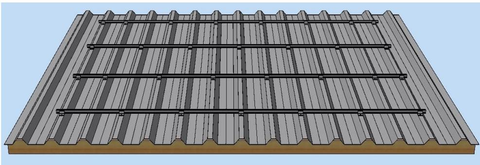
Figure 65: Mount carrier rail
