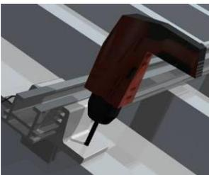
Figure 66: Drilling clamps
