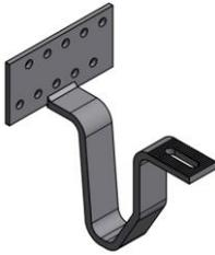
"Mammut XL S+" roof hooks are used to ensure the safety of the structure under very high snow loads. This roof hook provides improved static characteristics compared with the "Mammut S+" roof hook. In certain conditions (e.g. low snow load zone), it may be possible to install "Mammut XL S+" roof hooks only on every second rafter and consequently reduce the number of roof hooks. The load-bearing capacity of the substructure must be given special consideration.
