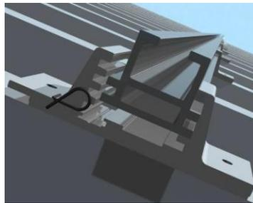
Figure 63: Align the carrier rail
