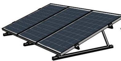
Figure 133: Delta support with single base rail
