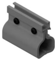
The clamps are mounted vertically according to the number of modules or carrier rails. As a rule, fit one standing seam to each clamp. On each side the carrier rail must protrude by a maximum of 0.4 m. Observe the thermal separations of the profiles after 3.3m or the specifications of the respective sheet seam manufactures.
