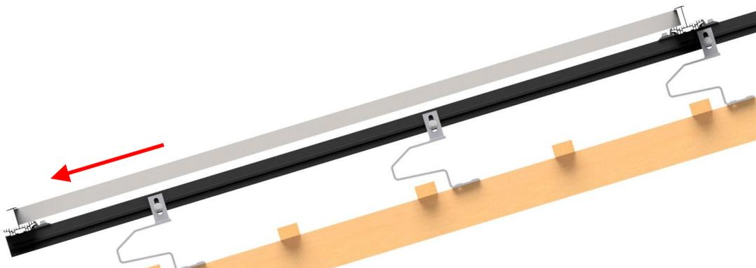
Figure 159: Slide module into position
