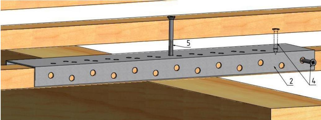
Figure 40: Fastening the batten rail
