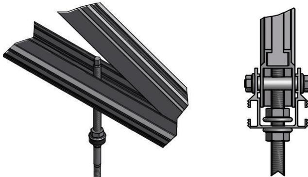
Figure 137: Fixation by hanger bolt
