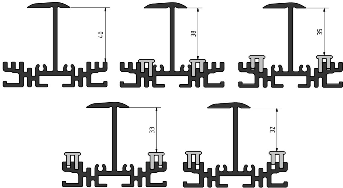
Figure 155: possible module frame heights
