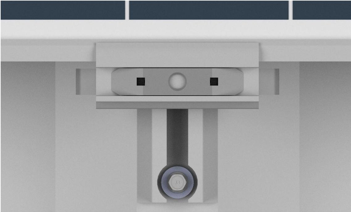
Figure 110 Place the clamps on the center of the Trapezoidal System Eco 120mm
