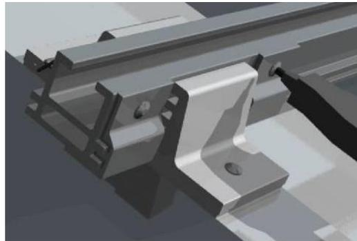
Figure 73: Rivet transverse securing clamps
