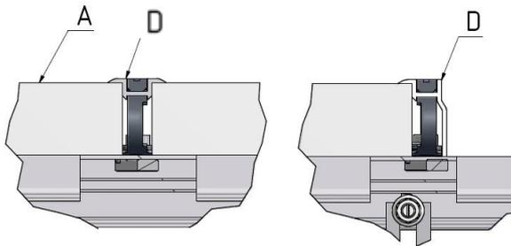
Figure 3: Module fastening of the IBC TopFix 200 pitched roof mounting system
