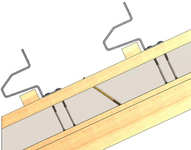
Figure 35: Roof hooks on rafter-mounted insulation systems
