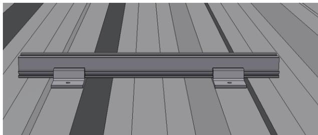
Figure 96: Affixing the "Trapezoidal System Eco"
