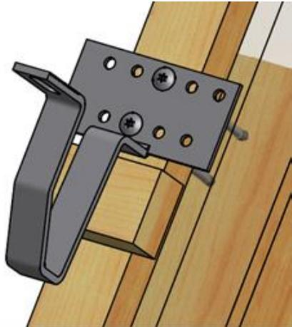
Figure 36: Inserting flat head screws
