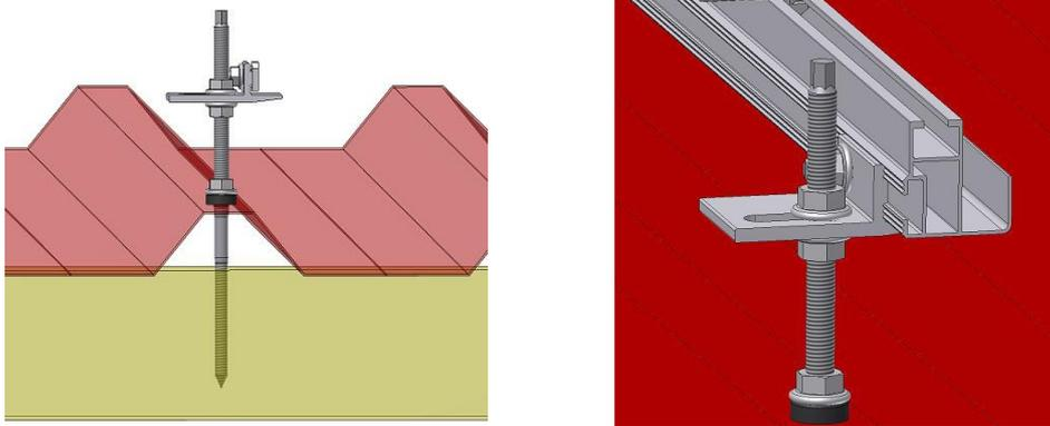
Figure 51: Correctly fitted hanger bolt with universal connector
