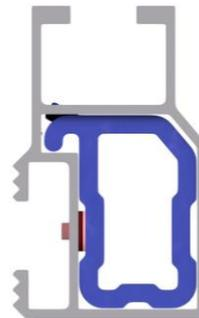
Figure 122: Butt connector TF50 + / TF50+m inside (blue) and leaf spring for potential equalization (red)
