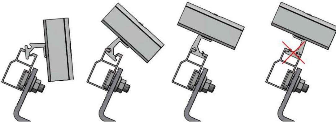
Figure 125: Inserting middle clamps G4
