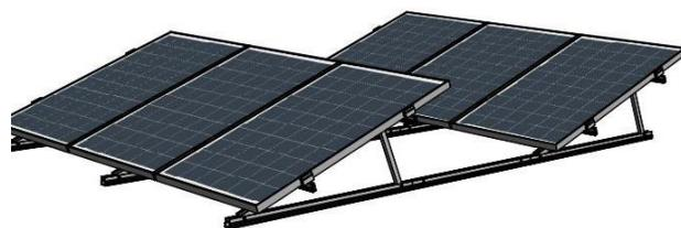
Figure 134: Delta support with continuous base rail
