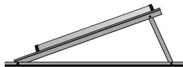
In this assembly process, modules are mounted directly on the Delta support. In this case, no further carrier rails are used. However, two Delta supports are required per module.
