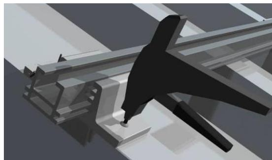
Figure 68: Riveting using a standard rivet head
