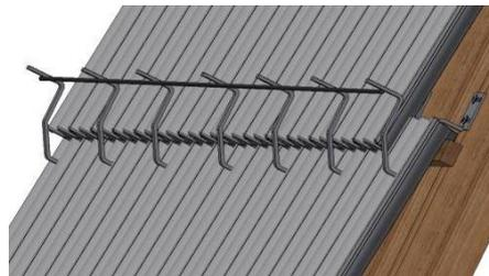
Figure 9: Alignment with piece of string
