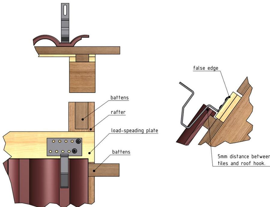
Figure 10: Roof hook load distribution
