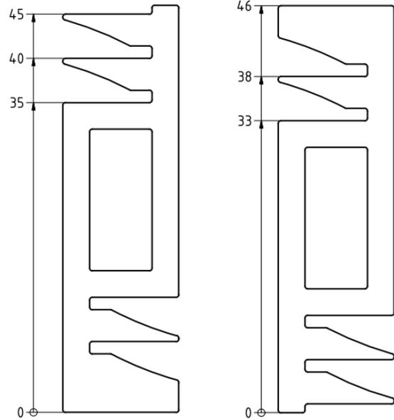
Figure 127: EC adapter frame heights
