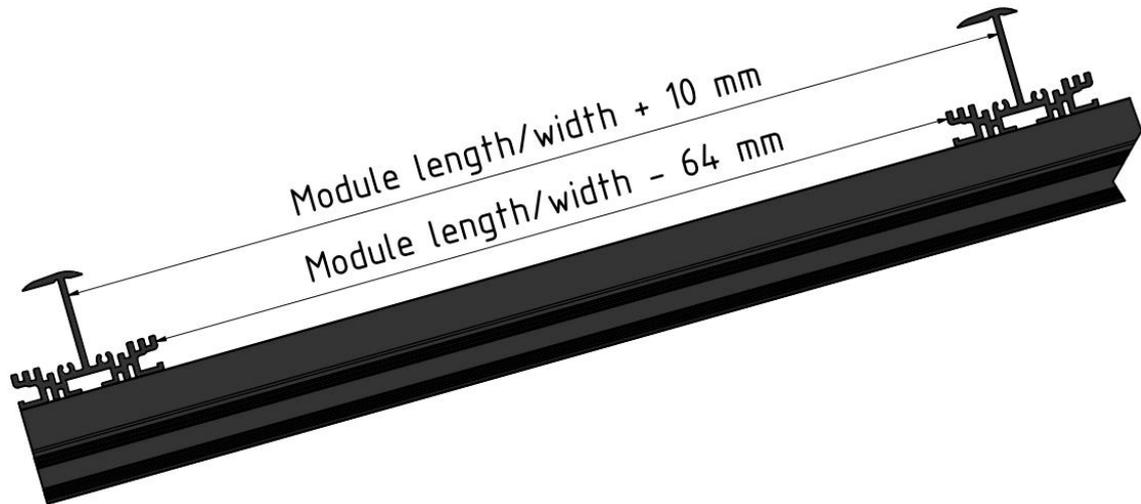
Figure 146: Insertion rails distance: Module length / -width + 10 mm, or module length / width - 64 mm
