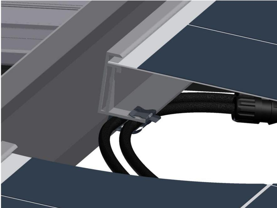
Figure 128: cable clip 0° on module frame
