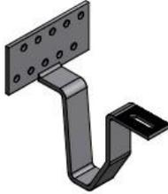
"Mammut S+" roof hooks are used to ensure the safety of the structure under high snow loads. This roof hook provides improved static characteristics compared with the "Standard S+" roof hook. In certain conditions (e.g. low snow load zone), it may be possible to install "Mammut S+" roof hooks only on every second rafter and consequently reduce the number of roof hooks. The load-bearing capacity of the substructure must be given special consideration.
