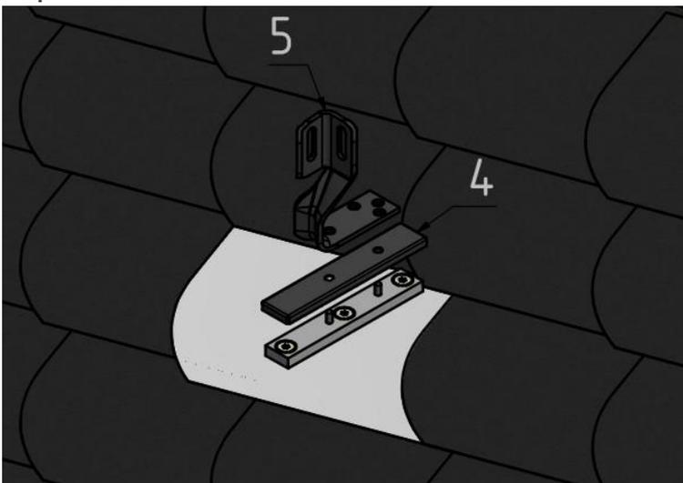
Figure 48: Roof hook fixing
