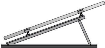
In this case, Delta supports are connected using two carrier rails (TF50+TF50+m/TF60). Modules are then mounted on said carrier rails.
