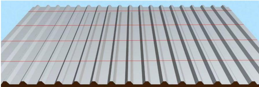
Figure 104: Marking fixing points
