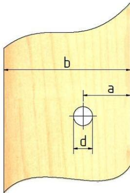
Figure 171: Defining the distance to the edge of rafters
