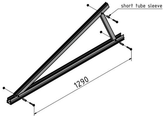
Figure 135: Assembling Delta supports at the base rails
