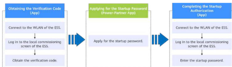
Figure 3-22 ESS startup authorization procedure
