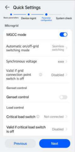
Figure 3-38 Microgrid configuration parameters (seamless PV+ESS networking)
