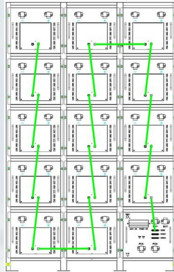
BR100 Battery Rack communication line installation diagram
